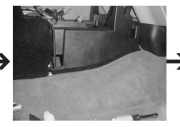
**STEP 28:** Attach the suppled backing loop tape to both bottom edges of the modified back inner console.
